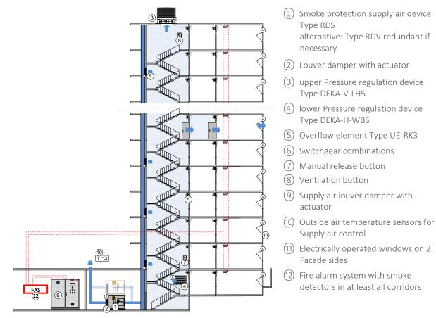
If an air release via the façade is planned within a pressure differential concept, the principle of thermal compensation can be applied. The influence of the thermal lift is compensated by the pressure loss during the perfusion of the stairwell.
