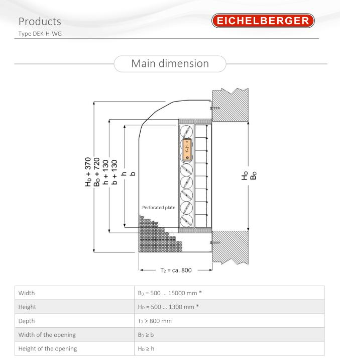
\* The maximum dimensions depend on the proportion  $H_D$  to  $B_D$  (see selection table). The area highlighted in grey in the selection table may be available with an enlarged overall depth  $T_2$  on request.
