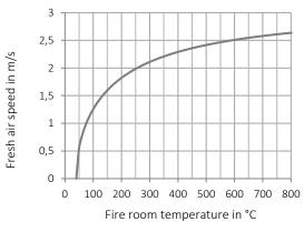
Figure 1: Fresh airflow rate through a 2m high and 0.9m wide door as a function of fire room temperature; John, R.
