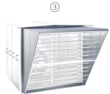
Aspiration ports made of galvanised sheet steel with integrated bird protection grid
