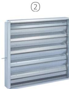
Insulated louver damper with spring return motor, 24 V, opens without electricity, mounted on the suction-side
